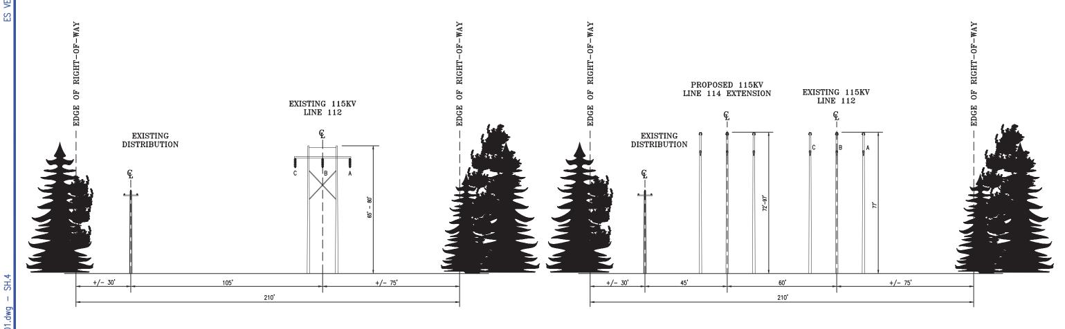
EXISTING CONFIGURATION: SINGLE CIRCUIT H-FRAME STRUCTURES (WOOD)
